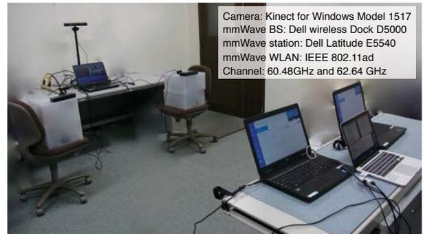
Figure 4: Our current testbed setup to study proactive handover in mmWave-Camera VLC systems
