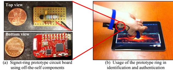
Figure 1: Ring Prototype
