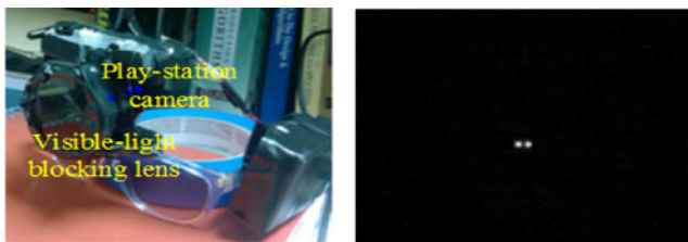
Image output of the IR camera (white blobs correspond to light output from a tag)
